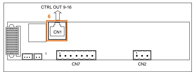
6 Connect CN1 (of rear left side) to CTRL OUT 9-16 of the VX-2000 (use Cat5/5E/6 FTP or STP or SFTP (with shield)
